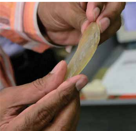
This 2-millimeter-thick polymer has shown early promise as a way to decrease the risk of concussions.
