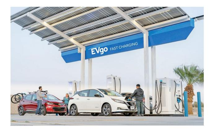
Bob Stojanovic, head of EV charging infrastructure for ABB in North America, said there are practical considerations in the race toward faster charging times. Not many vehicles can charge at 150 kW, and many are still at 50 kW and 75 kW. So 100-kW chargers will likely be the most common until more vehicles arrive that can utilize higher rates.
